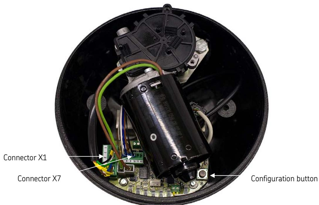
**Figure 2** Circuit board, EP-Co
