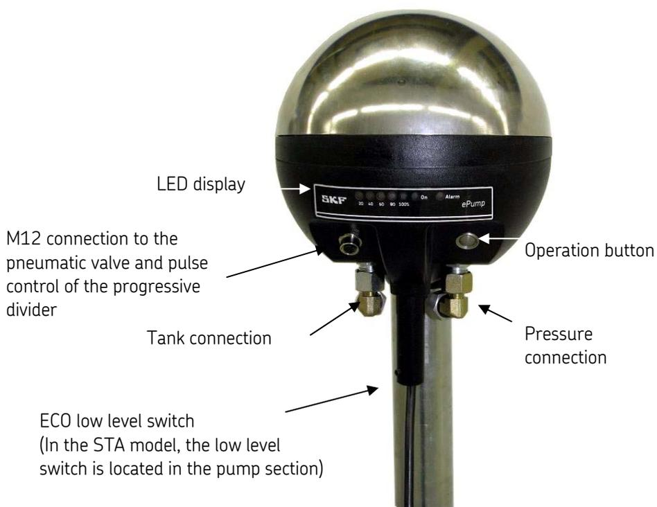
**Figure 1** Pumping unit SKF-EPUMP-XX-XXX-24-P
